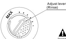
The rinse aid dispenser has six or four settings. Always start with the dispenser set on "4". If spots and poor drying are a problem, increase the amount of rinse aid dispensed by removing the dispenser lid and rotating the dial to "5". If the dishes still are not drying properly or are show spots, adjust the dial to the next higher lever until your dishes are spot-free. The recommended setting is "4". (Factory value is "4".)
